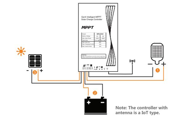
**B. Wiring diagram of the controller with external IoT module**
